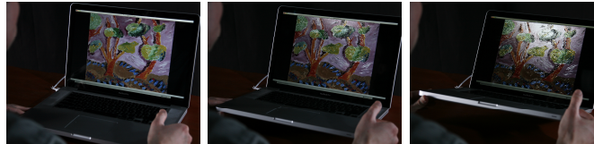
Tilting the laptop causes changes in virtual surface reflections, based on the new orientation relative to virtual lighting.
