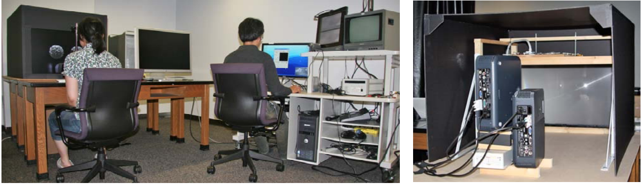
Figure 3: Experimental set up: (left) front view of HDR display showing LCD panel and adjacent eye tracker system, (right) rear view of HDR display showing tiled DLP projectors.
