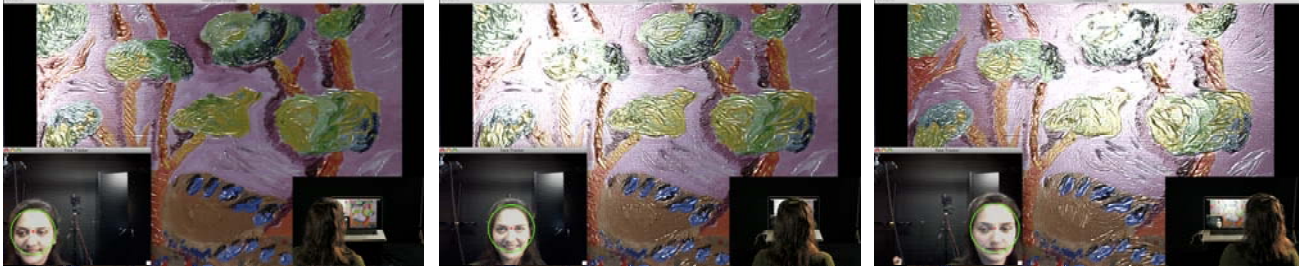
Figure 2: Image sequence illustrating the dynamic viewpoint control capabilities of tangible display systems. The insets show the observer's position (lower right) and the output of the head-tracking software (lower left) as the observer moves in front of the screen. The large images show the corresponding movement of the rendered surface reflections.
