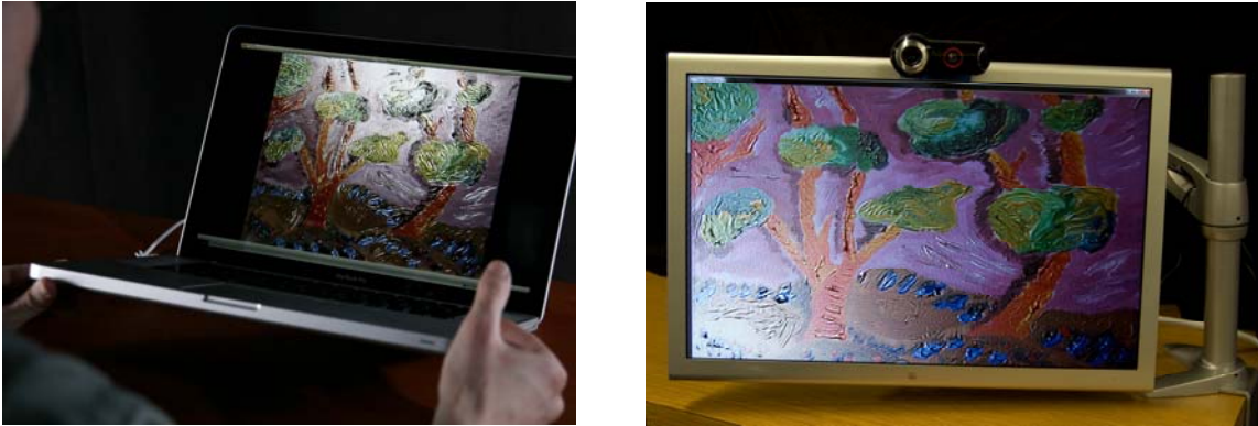
Figure 4: Tangible displays are being developed for two different architectures. Left, the first-generation tangiBook was developed from an off-the-shelf laptop computer. Right, a second-generation prototype is being developed using a desktop computer, external tracking devices, and an Apple Cinema HD display.
