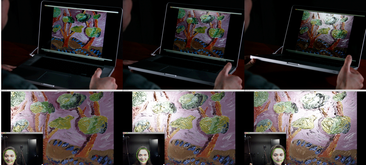
Figure 3: Image sequence showing a painting model being displayed on the tangiBook. The tangiBook is based on an off-the-shelf laptop computer that incorporates an accelerometer and a webcam as standard equipment. Custom software allows the orientation of the laptop screen and the position of the observer to be tracked in real-time. Tilting the laptop (as shown) or moving in front of the screen produces realistic changes in surface lighting and material appearance.
