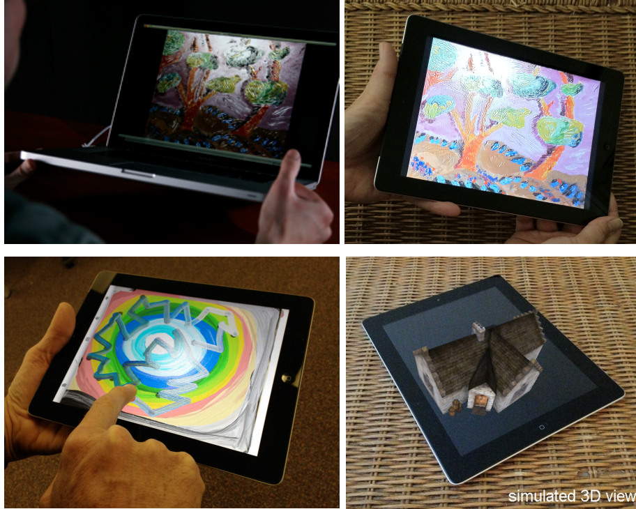
Fig. 1. Tangible imaging systems (left to right, top to bottom): The first generation tangiBook system developed using an off-the-shelf laptop computer; the tangiView system implemented on a tablet device; the tangiPaint application that allows direct creation of and interaction with rich digital paintings; the phantoView system that allows tangible interaction with three-dimensional object models.
