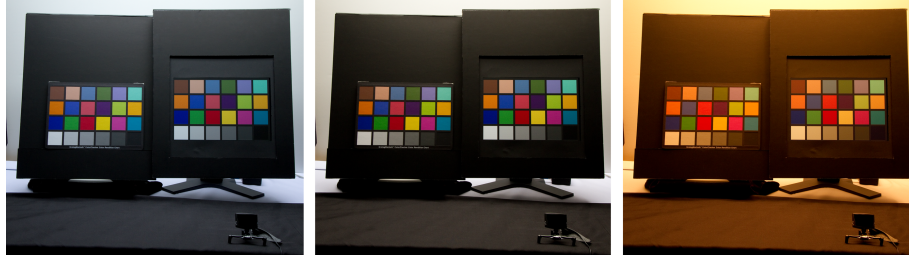
Fig. 7. Simulating color. In each panel the real Macbeth Color Checker Chart is on the left, the image produced by the system is on the right. Note that the simulated colors change appropriately with respect to the different illuminants.
