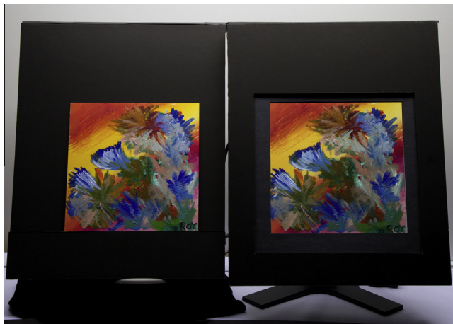
Fig. 1. A real painting (left), and a representation rendered by our surface display system (right). The color, gloss, and texture properties of the painting are all rendered correctly for the real scene lighting, and the appearance of the surface changes appropriately with movement of the observer or display.
