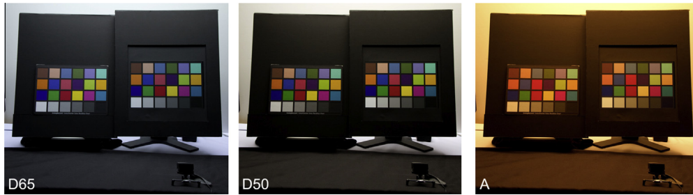
Fig. 11. Simulating color. In each panel the real ColorChecker chart is on the left, the image produced by the system is on the right. Note that the simulated colors change appropriately with respect to the light sources. The Supplementary video shows that the changes occur automatically and in real-time as the sources are switched.
