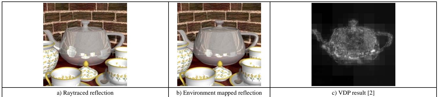
Fig 1. Images rendered with different reflection algorithms and VDP map showing areas of visible difference.
