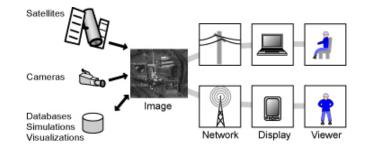
**Figure 1.** In heterogeneous networked display systems participants collaborate using systems that include four components: images captured from different sensors, networks, displays and viewers.
