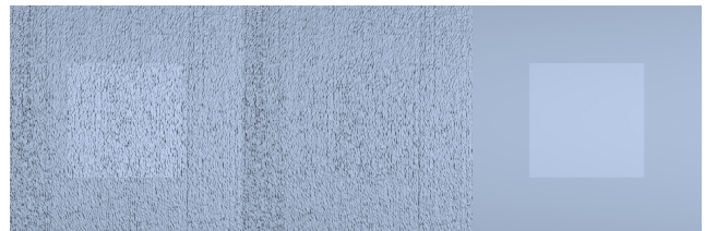
Figure 13. Contributions to the touch-up problem. Texture and BRDF differences (left), texture differences alone (center), BRDF differences alone (right).
