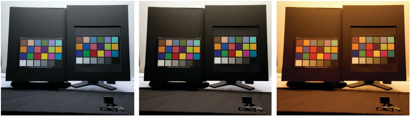
Figure 6. A sequence of images illustrating the system automatically updating the color of a virtual ColorChecker (right side) to continue to match the color of the real ColorChecker (left side) as the light changes between the D65 light (left image), D50 light (center image) and tungsten light (right image). The images were purposely not color balanced (all were set to a CCT of 5500) in order to clearly show the changing illumination.
