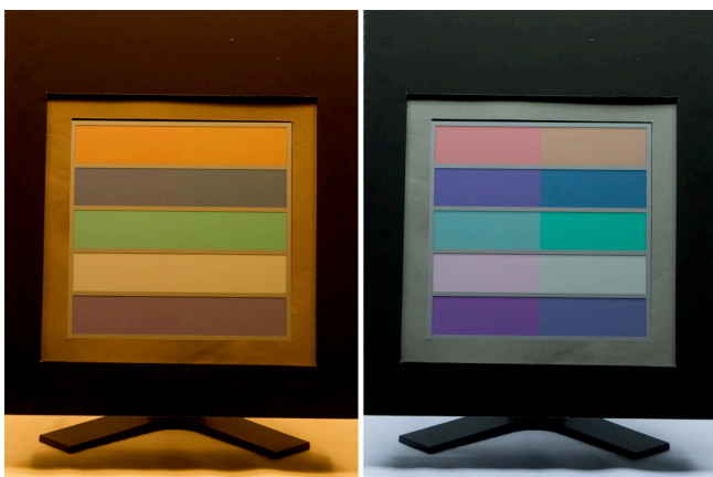
Figure 7. A set of metamerism samples displayed under the tungsten light (left) and the D65 simulator light (right). Each row of the target contains two virtual samples with spectra that were selected to provide a metameric match under the tungsten light and a color difference under the D65 booth light.
