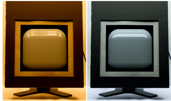
Figure 5. Left, the virtual reflection of the tungsten light booth source on a virtual curved surface. Right, the virtual reflection of the D65 source. Based on a spectral classifier, the system automatically identifies which light is present and switches the spatial light map used to calculate the reflections.
