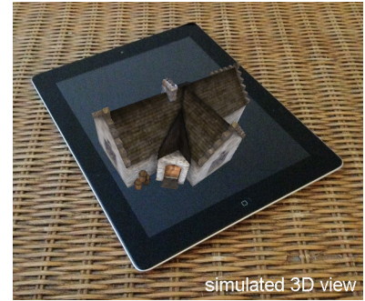
Figure 6: The phantoView system – 3D object models loaded into the system are rendered in real-time as phantograms to the tablet's display. A rendered object appears to be sitting on the tablet's surface. Rotating the tablet about the vertical axis allows the object to be seen from other viewpoints.
