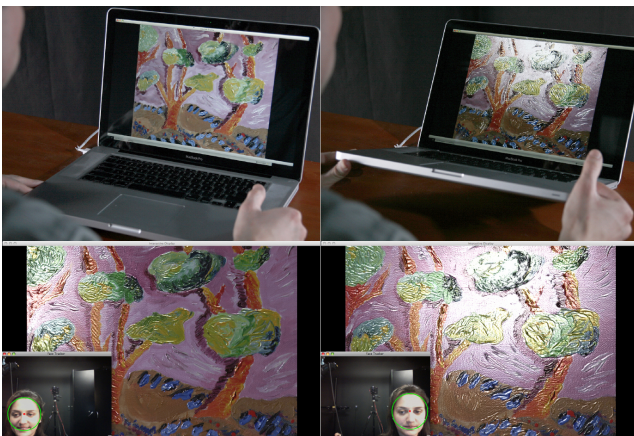
Figure 2: The tangiBook system – tilting the display (top row) or moving in front of it (bottom row) produces realistic changes in the appearance of the rendered surface.
