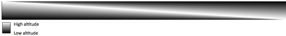
Figure 1. Height map of twisted target, which is to be printed by the wet-on-dry printer.
