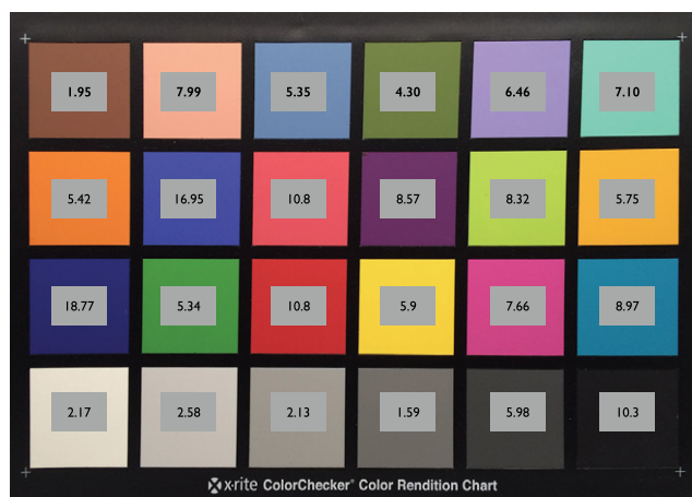
Figure 3. Testing the accuracy of the diffuse reflectance estimation method. Insets show the \Delta E_{ab} color differences with respect to ground truth.
